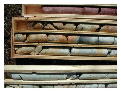
Illustration 1: Drill core from the Kiggavik deposit, Nunavut, illustrating the gradation from hematite alteration (red) through bleach clay alteration (biege) to deposition of uraninite (a uranium mineral, black).
