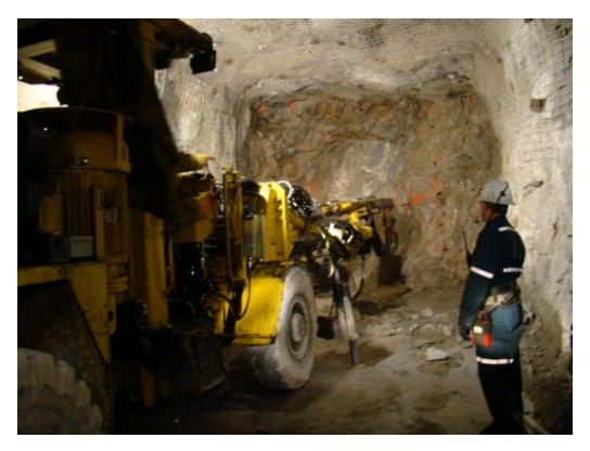
Fig. 4. Mechanized drilling at the Rabbit Lake underground mine. (Photograph by A. Liu, DFO)
