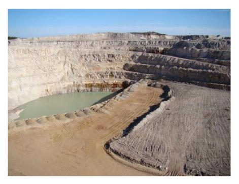
Fig. 6. Waste rock disposal at mined-out open pit at McClean Lake. Potentially acid-generating rocks are disposed of under water while non-acid-generating materials with low radioactivity are placed dry under a till cover.
